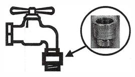
Another method of preventing backflow with a garden hose is using a device known as a vacuum breaker. Vacuum breakers are inexpensive devices that can be screwed onto your outside faucet. These devices will prevent contaminants from being siphoned back into your plumbing and the public water system.
